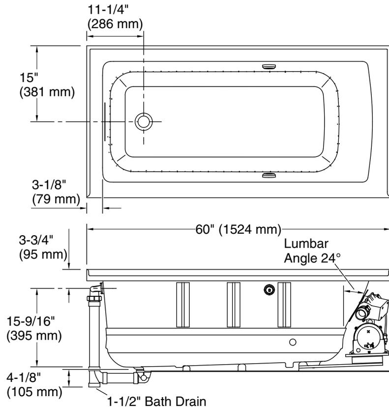
No change in measurements if connected with drain illustrated. (K-7272)
